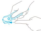
**Concealed blade – a maximum degree of safety** The SECUMAX 350 blade is not an open one, but is hidden from people and goods. This provides you with a maximum degree of safety from cut injuries and from damage to goods.
