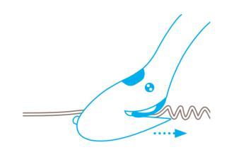
The **plastic guide** flattens the material being cut, making thin foil and paper easy to work with.
