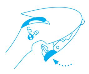
Finally, close the blade cover and push the blade holder **back into the handle**. With a click, everything is in place.
