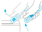
Automatic blade retraction – a high degree of safety The automatic blade retraction of the SECUNORM PROFI25 MDP guarantees a high degree of safety from cut injuries. As soon as you have started to cut, take your thumb off the slider. Then the blade will retract into the handle immediately after leaving the material being cut.
