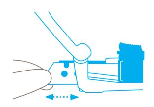
Now either rotate or change the blade, before pulling the blade carrier back into its original position.
