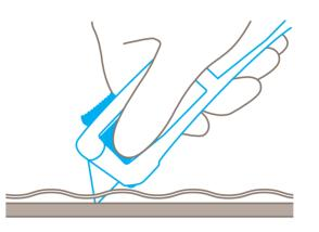
When cutting film, be sure there is **enough counter-pressure** that the blade does not retract by itself.
