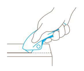
To engage the blade, unlock the cutter and **squeeze the lever**. Now you can cut.
