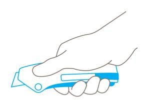
To **engage the blade**, unlock the cutter and squeeze the lever. Now you can cut.
