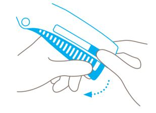
Swing the lever completely **out of the handle**, Now you can either **rotate or replace** the and flip open the blade cover.
