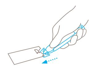
Use the small scraper at the head of the cutter for **light scraping work**: e.g. to remove labels.
