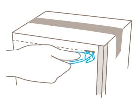
Pierce into the cutting material using either side of the cutter head.
