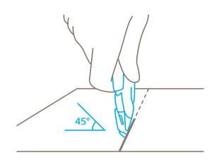
Hold the cutter at a **slight angle** when cutting open cardboard boxes.
