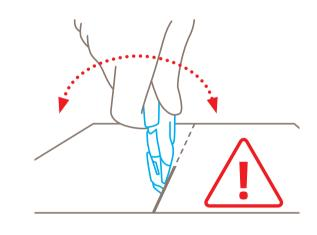
If the blade head becomes stuck, **don't** forcefully lever the cutter!
