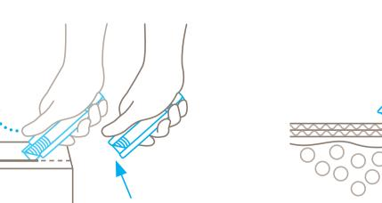
Following cutting, the blade immediately retracts into the handle. Condition: you have to protect your goods. released hold of the slider.
