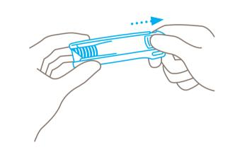
Press the blade-change button and **pull out** The blade cover opens **automatically**. the plastic insert.
