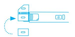
Reverse or replace the blade. Make sure you Finally, re-insert the slider and blade **fully** position the blade **exactly** over the location into the handle.
