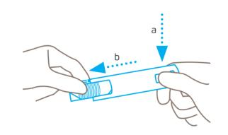
Press the blade change button downwards and at the same time pull out the slider all the way from the front.
