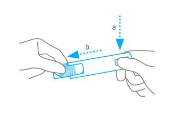
Press the blade change button downwards and **at the same time** pull out the slider all the way from the front.
