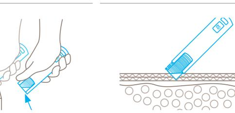
Following cutting, the blade immediately retracts into the handle. Condition: you have released hold of the slider.
