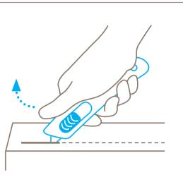
Position your **thumb** on the slider's grooved section.
