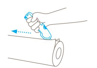
For **power cutting**, rotate the knife in your hand, push the lever and move it forwards with a high degree of pressure.
