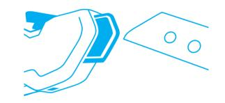
Now **reverse or change** the blade. Make sure that the blade is exactly positioned on the cams on the blade holder.
