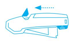
Pull the **blade change button** to the top and release the lever. Blade and blade holder will come out of the handle.
