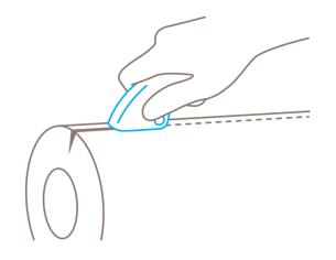
Use the underside of the knife head as a supporting surface to **work ergonomically** and efficiently.
