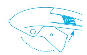
Finally, push the lever back into the handle until you hear it click into place.
