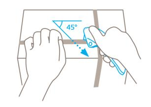
To engage the blade, unlock the safety knife and squeeze the lever. Now you can cut.
