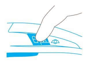
To prevent unintentional blade activation, always lock the safety knife by pressing downwards on the lock symbol.
